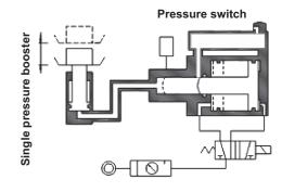
The booster can transform low pressure input to high pressure output in a efficient way.
