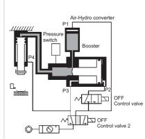
P2, a ram will advance. The high pressured fluid will come in to the hydraulic cylinder which will be goes back. forwarded by large thrust.
